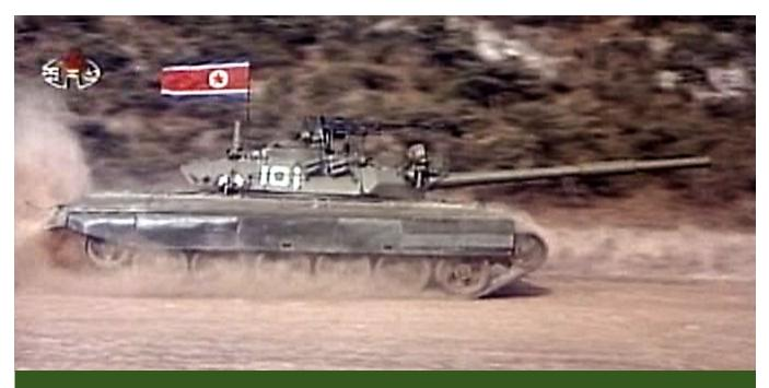
Vehicle #101. Note the missing from mud guard and the flexing side skirt panels. (Korean Central Television)
