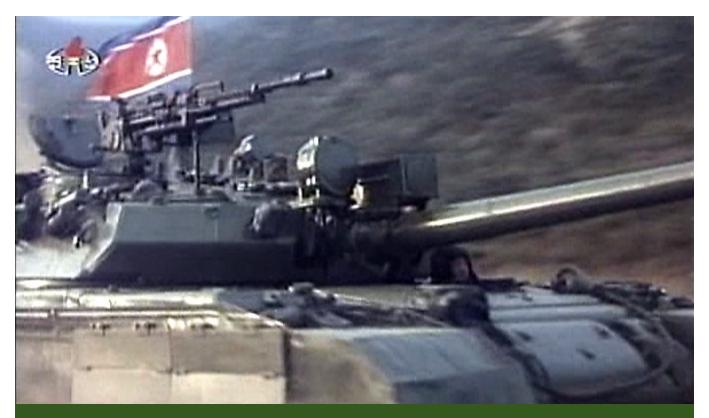
Vehicle #131. Close-up of the front end showing details of the turret front laminate module, glacis plate appliqué armor module, 14.5 mm machine-gun and laser range-finder. (Korean Central Television)
