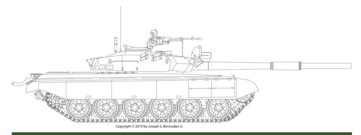
Provisional scale drawing of the P'okpoong MBT (2009), based upon available imagery. An precise scale drawing will have to wait until measurements can be taken of the vehicle. (Copyright © 2010 by Joseph S. Bermudez Jr.)
