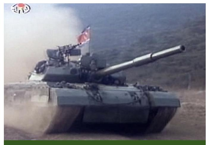
Vehicle #131. Note the tow cable on the glacis plate appliqué armor module and that the laser range-finder does not have a cover. (Korean Central Television)
