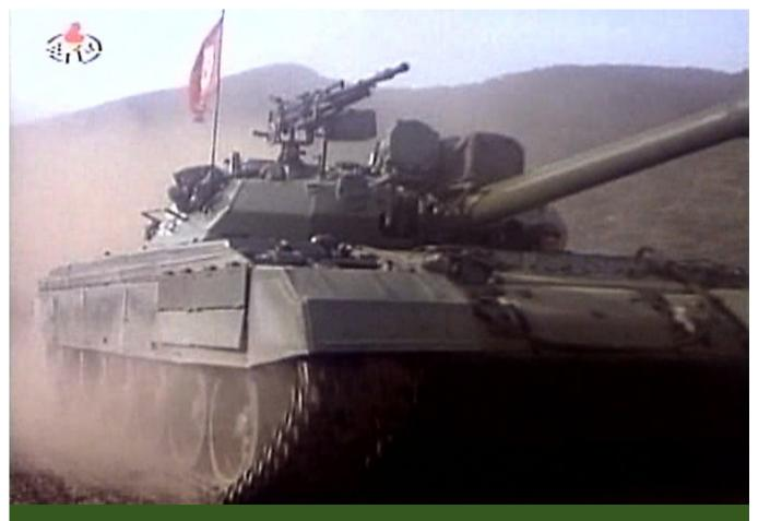
Vehicle #123. Visible in this image are the wedge-shaped laminate module on the front of the turret, glacis plate appliqué armor module, folding panels on the side skirt and laser range-finder (with cover) on the main gun. Note the driver on the left side of the tank as in the T-62. In the T-72 the driver sits in the center. (Korean Central Television)
