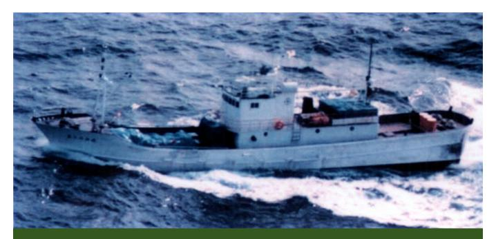
Views of one of the two DPRK infiltration vessels fleeing at high speed from JMSA and JMSDF vessels. Note how the specially designed hull allows the vessels to ride high and more easily slice through waves and swells. What appears to be the stern clam-shell doors to the internal "wet-well" are visible in the lower image. (Japan Maritime Self-Defense
