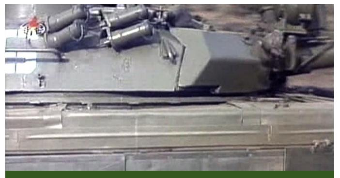
Vehicle #126. Close-up of the wedge-shaped laminate module and smoke discharges. (Korean Central Television)
